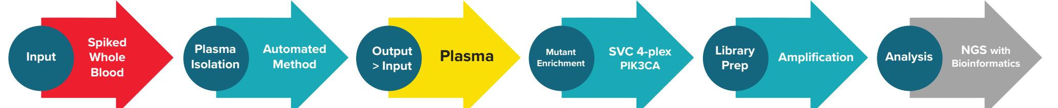
Figure 5. The DNAe in-development automated NGS workflow (teal arrows) with orthogonal sequencing (gray arrow): from whole blood to bioinformatics report.
